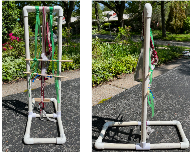
Figure 5. Front and side views of my PVC version of the Cranach loom.
