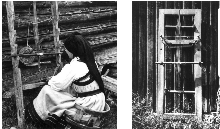
Figure 4. Two traditional Norwegian band looms recorded by Anna Grostøl. a. Weighted warp (Grostøl, 1939). b. Warp beam (Grostøl, 1935).
