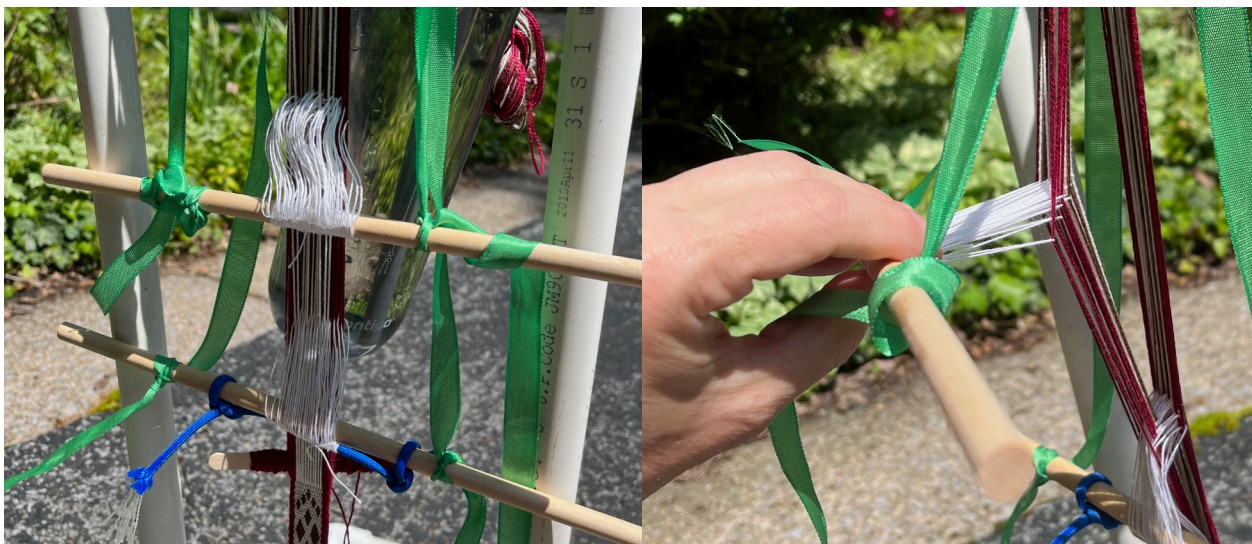
Figure 6. Heddle bars on my PVC version of the Cranach loom.
